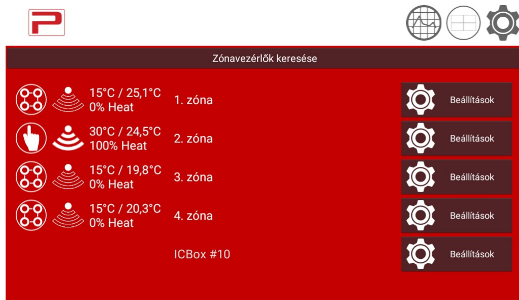
Figure 23.: Unassigned IC-BOX in the Zone list
