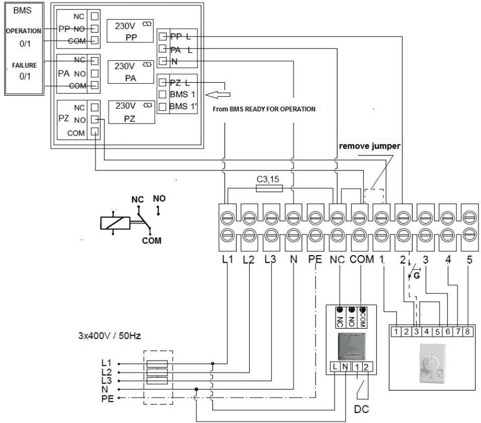
**ATTENTION ! While using BMS communication module for ACR electric series remove factory installed jumper between COM-1**
