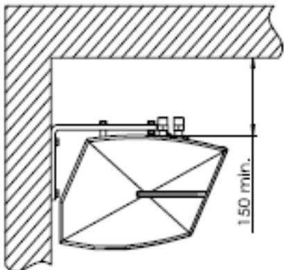
Wall installation by means of a horizontal brackets
